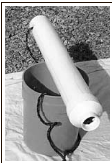
Bottom end; tank ball visible in opening.
